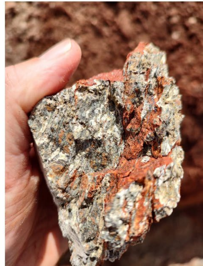
Figure 2: Photographs of trench TR22TR01 at Tróia target (top picture, looking east), with trench wall sampling intervals (bottom center and bottom left pictures) and a sample of chromitite-rich ultramafic rock submitted for PGE assay (bottom right picture).
