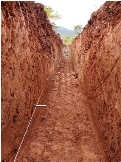
Figure 2: Photographs of trench TR22TR01 at Tróia target (top picture, looking east), with trench wall sampling intervals (bottom center and bottom left pictures) and a sample of chromitite-rich ultramafic rock submitted for PGE assay (bottom right picture).
