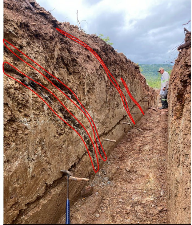
TR22TR02 - 26 m @ 0.82 g/t 2PGE+Au Multiple centimetric Cr reefs (red) within Cr-rich UMs
