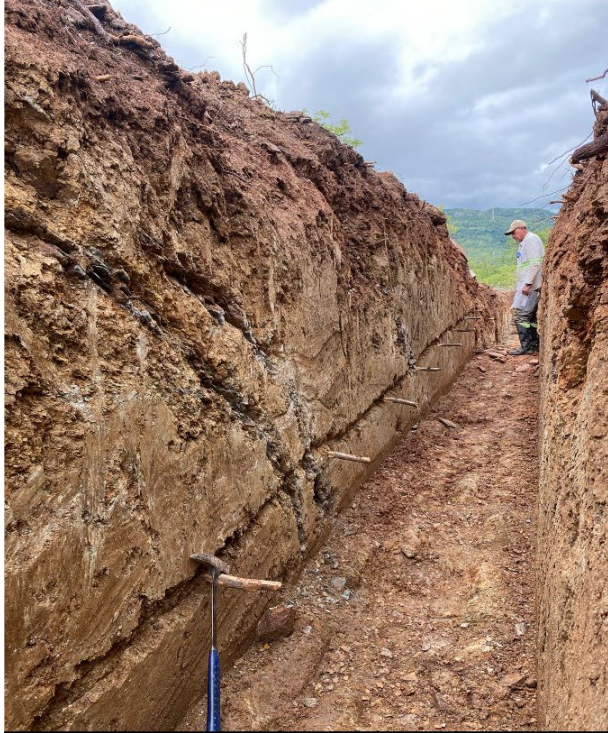
TR22TR02 - 26 m @ 0.82 g/t 2PGE+Au Chromitite-reefs within Cr-rich UMs - dipping E
