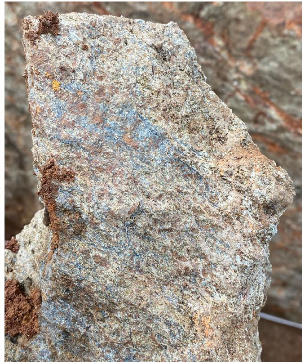
TR22TR03 - Chromite-rich peridotite within 42 m @ 0.87 g/t 2PGE+Au
