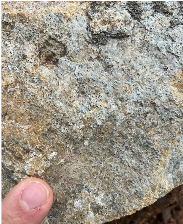
TR22TR02 - Chromite-rich serpentinized UM 2.60 g/t 2PGE+Au sample
