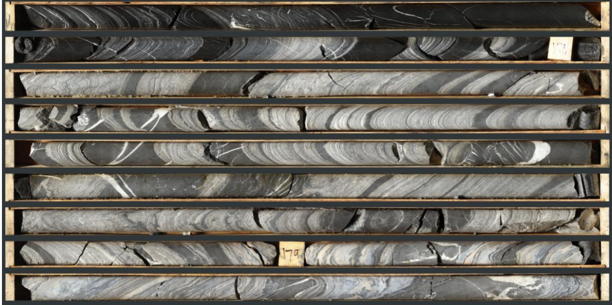
Photo 3: High resolution core scanning image of barite-sphalerite-galena stratiform mineralization in black, grey and pink facies from TS23-007 (170.9 m to 180.6 m)
