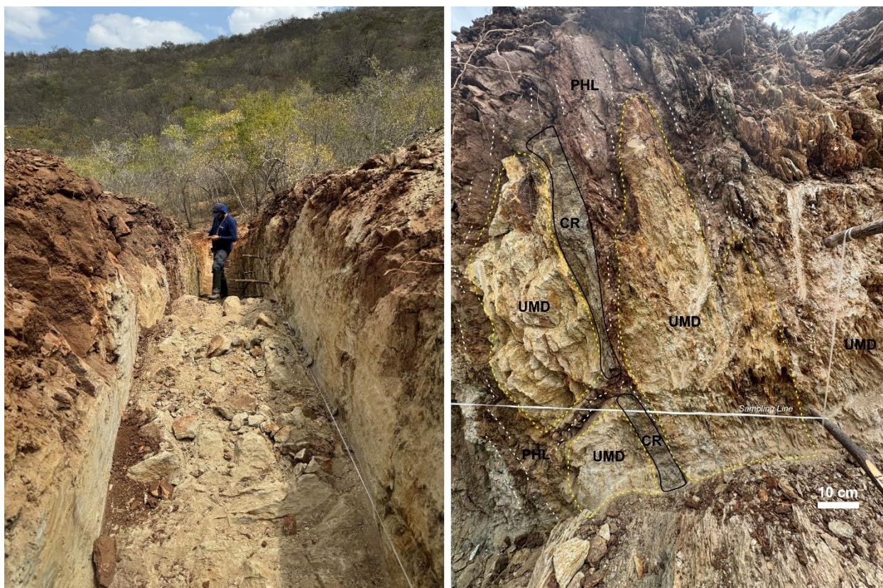
Figure 2: 2024 Salvador trenching program. Mapping and sampling of trench TR24MES06 (left), and centimetric chromitite layer (CR) within serpentinized ultramafics (UMD) and phlogopite (PHL) (right).
