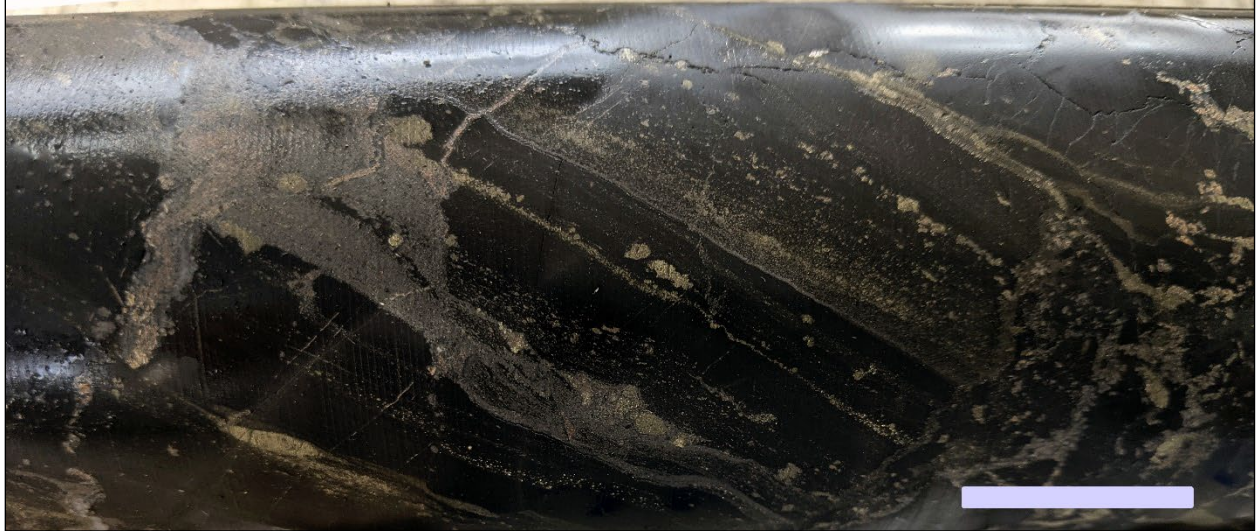
Photo 1: Illustrating laminated high-grade mineralization from the stratiform zone: grey sphalerite and brassy pyrite within black mudstone cut by pink sphalerite veinlets. From NB21-009, 241.5 m depth, scale bar 20 mm.
