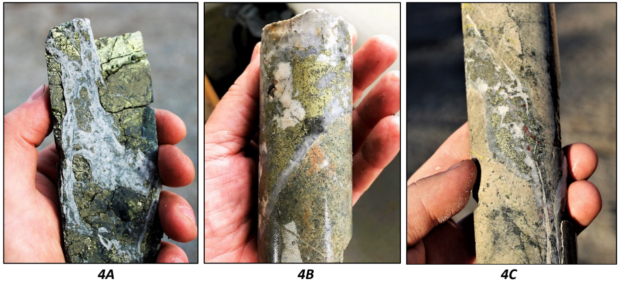
Figure 4: Examples of core from 2021 Drilling at MPD: 4A) MPD-21-018: Semi massive, chalcopyrite-pyrite in quartz-carbonate stockwork/breccia hosted in altered porphyritic andesite. Core is from a 126.0 metre intercept reporting 0.72% Cu, 0.21 g/t Au and 2.95 g/t Ag from 500.0 to 626.0 metres. 4B) MPD-21-026: Chalcopyrite-pyrite (+/-bornite) mineralization with quartz within phyllic-potassic altered, crowded feldspar-hornblende diorite porphyry. Core is from a 111.0 metre intercept reporting 0.53% Cu, 0.34 g/t Au and 1.84 g/t Ag from 563.0 to 674.0 metres. 4C) MPD-21-017: Chalcopyrite-pyrite-hematite mineralization with quartz-carbonate breccia/veining in intensely altered andesite displaying local phyllic overprint. Core is from an 81.0 metre intercept reporting 0.31% Cu, 0.13 g/t Au and 1.41 g/t Ag from 257.8 to 338.0 metres. Images are of selected intervals and do not represent all mineralization on the property.
