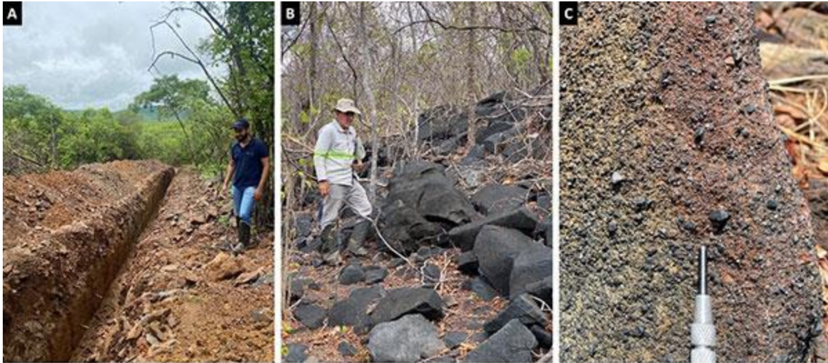
Figure 3: A. Overview of trench TR22IP01, totaling 71 m from northwest to southeast. B. Chromitite boulders marking an outcropping area of approximately 100 m along trend by 30 m wide crosscut by, and outcrop within, trenches TR22IP01 and TR22IP02. C. Detailed photograph of the high PGE grade chromitites.
