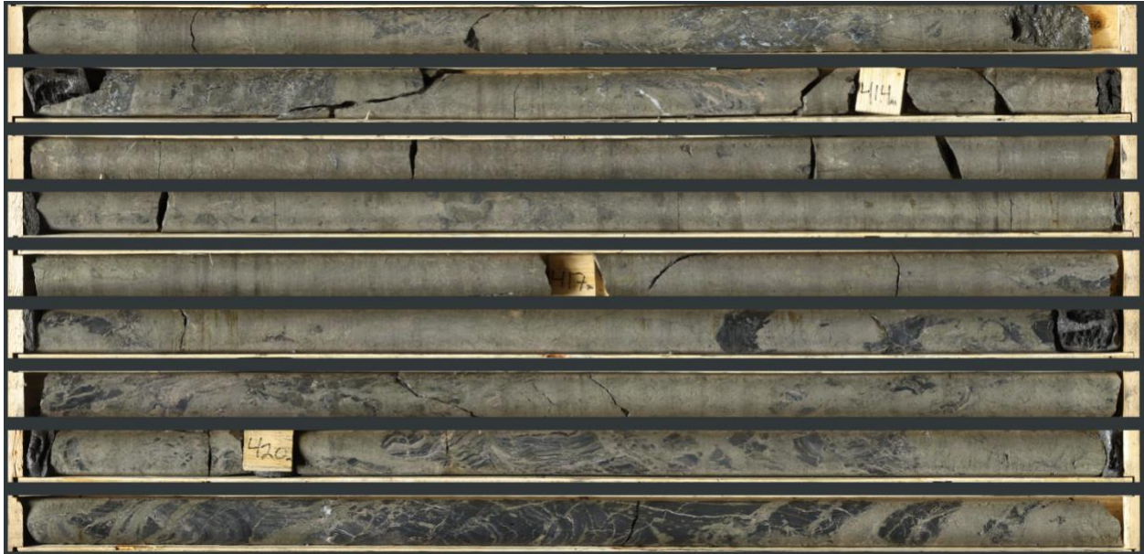
Photo 2: High resolution core scanning image stratiform and massive to semi-massive sulphide mineralization in NB23-037 (412.1 m to 422.1 m)
