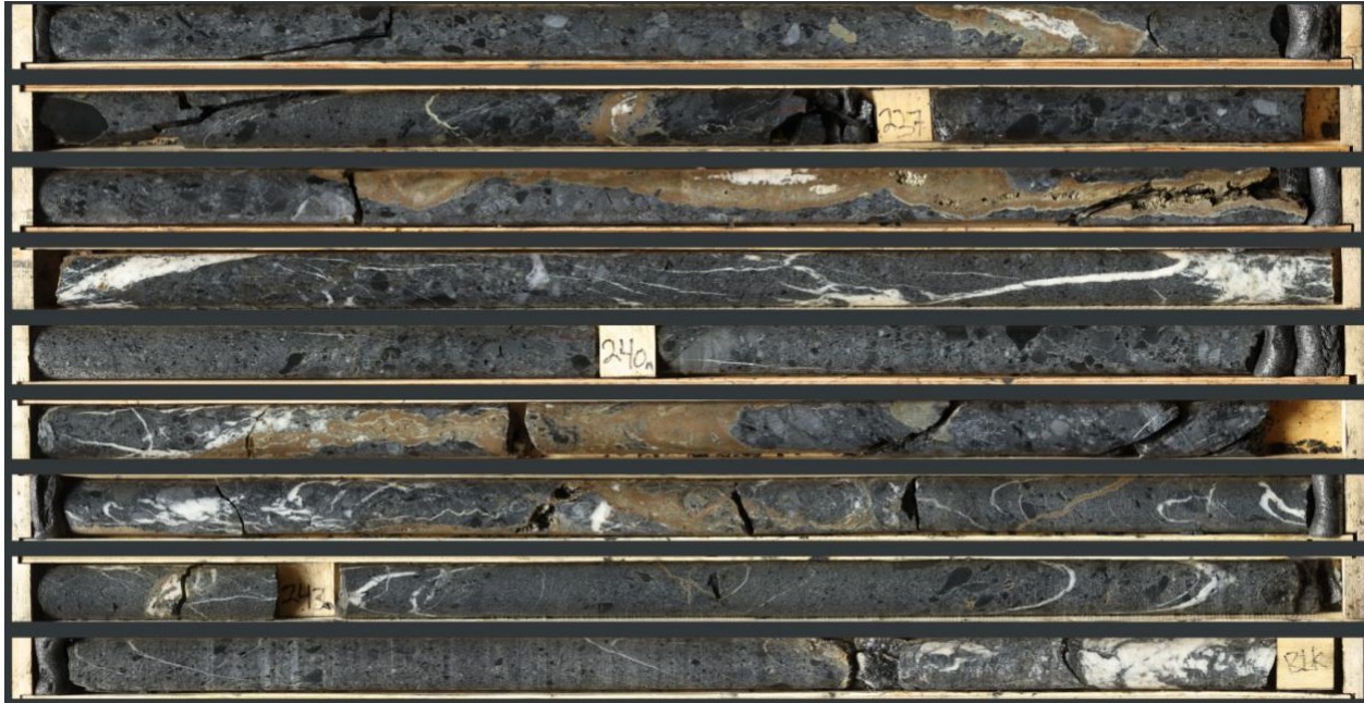
Photo 3: High resolution core scanning image of sphalerite-pyrite-siderite vein mineralization in NB23-037 (235.1 m to 244.9 m)
