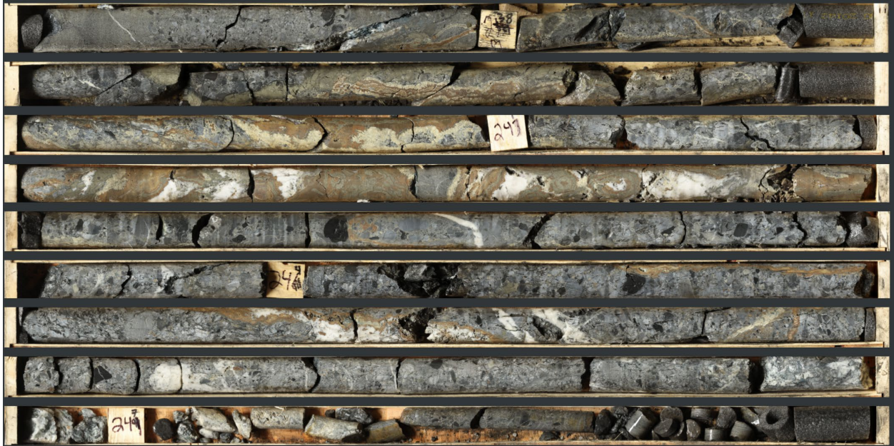
Photo 2: High resolution core scanning image of sphalerite-pyrite-siderite vein mineralization in NB23-029 (237.5 m to 247 m)
