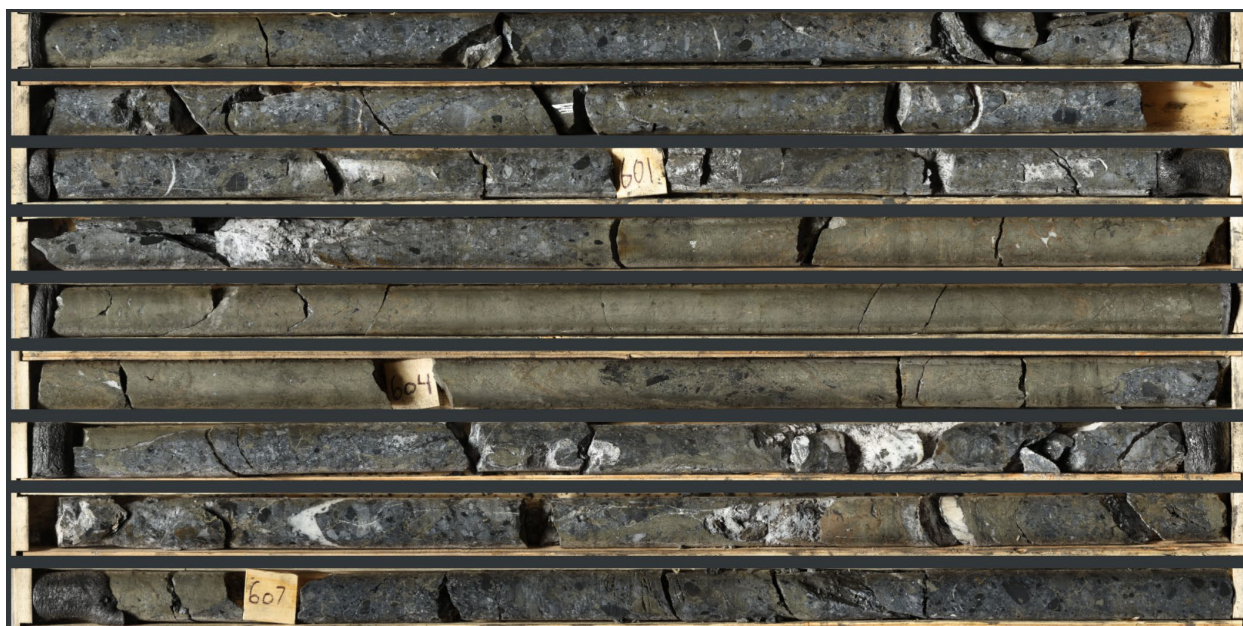
Photo 3: High resolution core scanning image of sphalerite-pyrite-galena-siderite breccia and massive sulphide mineralization in NB23-029 (598.4 m to 607.9 m)
