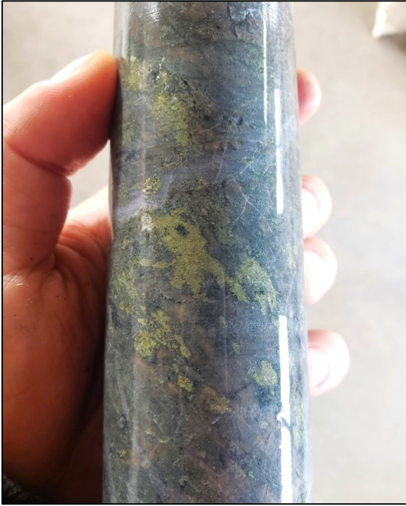
Figure 4: Core from 1516 Zone hole AXE-23-018 (left). Patchy epidote-pyrite-chalcocopyrite in brecciated intermediate altered volcanics with molybdenite in quartz veining at 729 m. Drilling at 1516 Zone (right).
