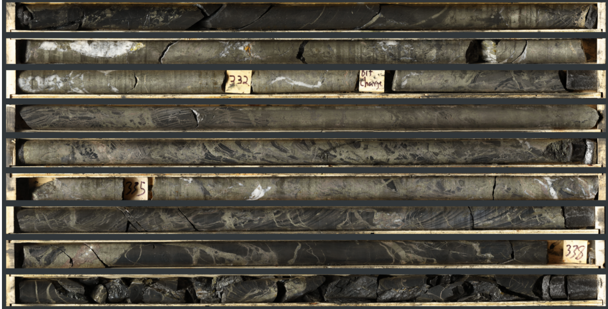
Photo 1: High resolution core scanning image of stratiform and massive to semi-massive sulphide mineralization in NB23-019 (329.4 m to 338.6 m).
