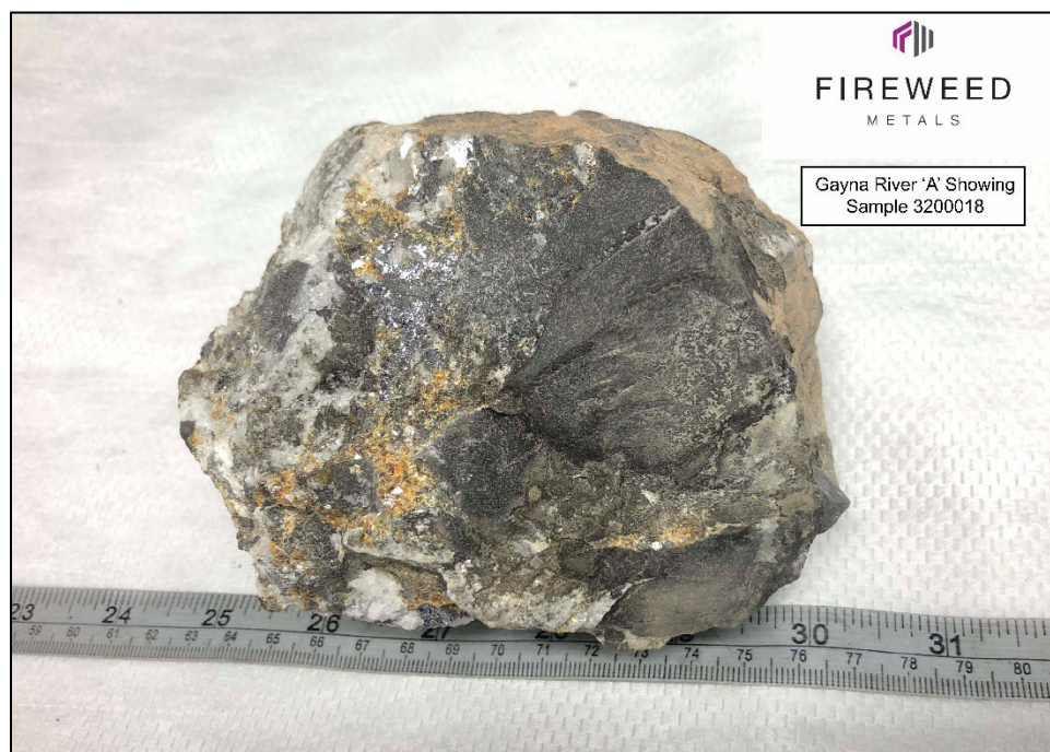
Photo 1: Gayna Project 'A' showing, sample. Upper-Host sub-rounded dolostone breccia, matrix infilled with dolomite, calcite, crystalline red and green sphalerite, and metallic galena.
