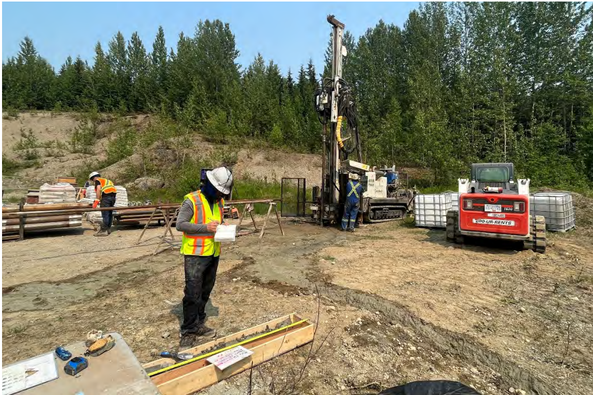
Image 1: SRK engineering personnel logging WSF sonic overburden material
