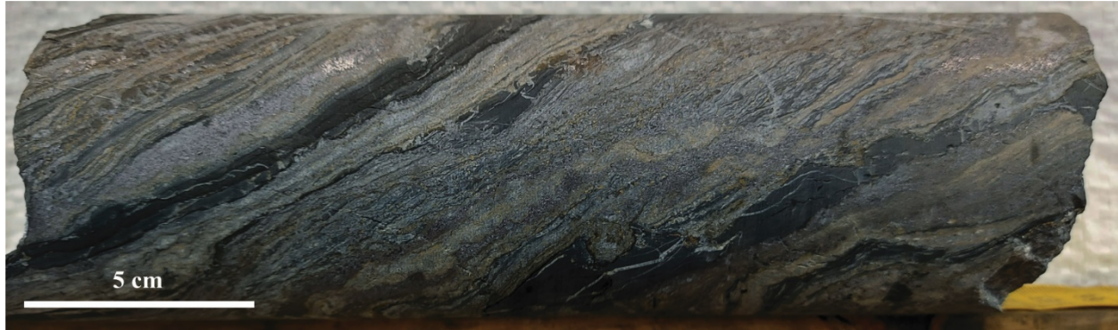
Photo 1: Hole TS21-001 at 148.53-148.73 m illustrating laminated high-grade mineralization.
